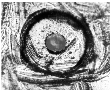
Figure 1-6. Damage from improper cleaning.
